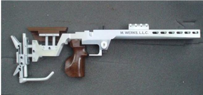
The tuner assembly in this stock should be handled with care until it is fully assembled. After full assembly into the stock the tuner is very robust and needs no more care than given to any fine rifle.
