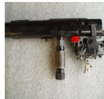
Note the orientation of the knob mark for the zero tune reference
