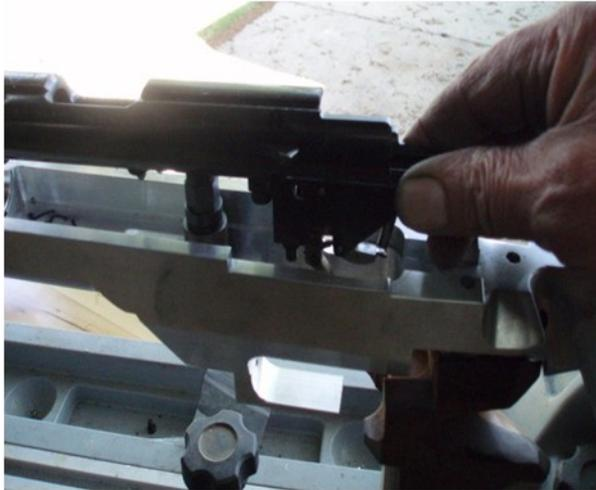
With the barrel located in the saddle tighten the side lock lightly until you are able to put the saddle top cap, including the sleeve, in place and start the 8 screws. Bring each of the 8 screws down to touch and check the gap between the cap and the stock to make sure it is reasonably even.
